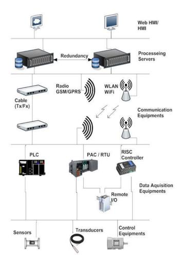
Fig. 1 - A Typical SCADA System Architecture [1]
