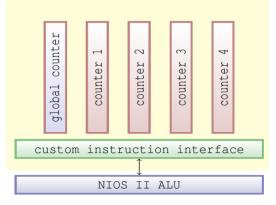
Fig. 1. Performance counter custom instruction block diagram.
