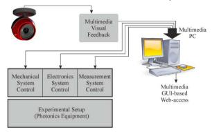
Figure 3. Web-based multimedia laboratory system.
