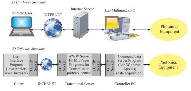
Figure 1. Web-controlled laboratory architecture.
