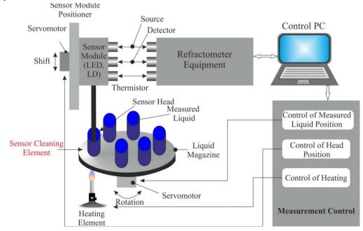
Figure 5. Web-controlled laboratory architecture.
