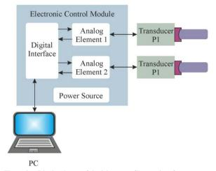
Figure 2. Block scheme of the laboratory fiber optic refractometer equipment.
