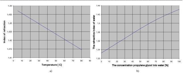
Figure 8. The refractive index of a) the propyle glycol vs. temperature (°C) and b) the water vs. propyle glycol concentration.
