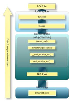
Figure 1. Data flow from physical layer to the libpcap-based capture application
