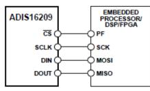
Figure 3: SPI communications with sensors
