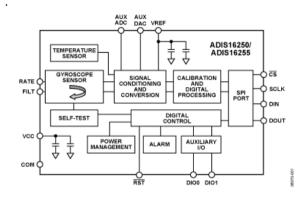
Figure 4. Gyroscop sensor functional block diagram
