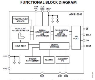
Figure 2: Functional block diagram ADIS 16209
