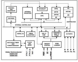
Figure 5. Functional diagram of DS89C450
