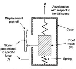
Figure 1. A simple accelerometer [5]
