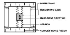
Figure 2. A simple Gyroscope [12]
