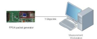
Figure 3. Custom FPGA-based packet generator is directly connected to the measurement workstation via a twisted pair Gigabit Ethernet link.
