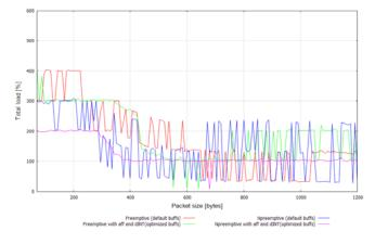
Figure 10. Aggregated CPU load in percentage at various packet sizes from 72 to 1200 bytes. Measurements were performed using both preemptive and non-preemptive kernels with and without the optimization method.
