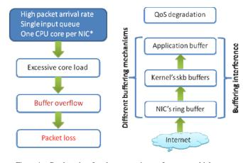
Figure 1. Bottlenecks of packet processing performance at high traffic intensity.
