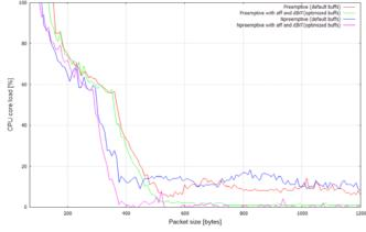
Figure 4. The CPU load of the softIRQ at various packet sizes from 72 to 1200 bytes. Measurements were done using both preemptive and non-preemptive kernels with and without the optimization method.
