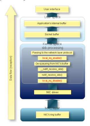
Figure 2. Interrupts are disabled on the dedicated CPU core while it executes the packet processing bottom-half handler.
