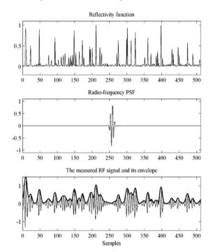
Figure 2. Simulated signals. Top: the generated reflectivity function. Middle: the generated PSF. Bottom: the resulted RF signal and its envelope.
