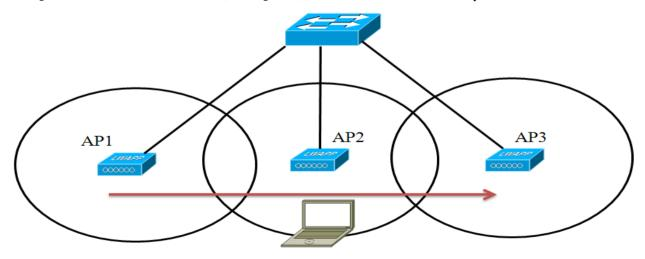
Figure 1. The L2 roaming process
