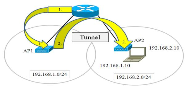
Figure 3. Packet transfer after L3 roaming
