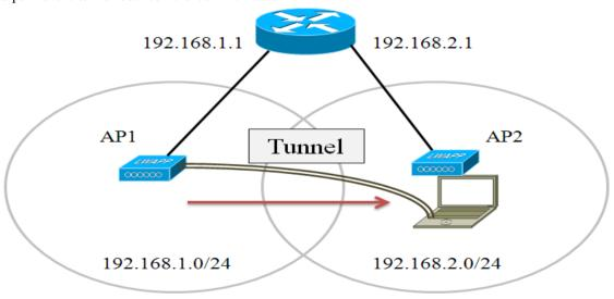
Figure 2. The L3 roaming process
