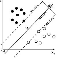
Figure 1. Hyperplane for a SVM trained with two classes. Samples on the margin are support vectors.
