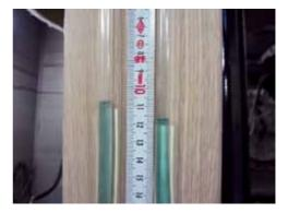
*Figure.11* Visual pressure drop measurement, *U-manometer.*
