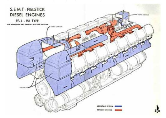
Figure.2 Air admission and exhaust system diagrams of PA4-185 diesel engine.[Semt Pielstick].
