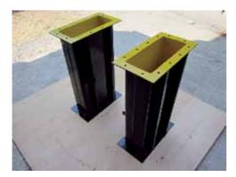
Figure.8 Manufactured distance units.
