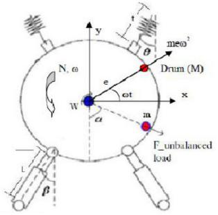
Fig.1 Physical model of the washing machine [9], [11].
