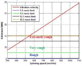
Fig.4 Vibration severity of the washing machine and Bernhard limits.
