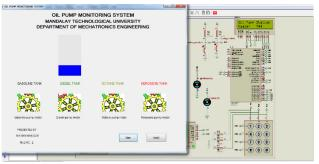
Fig.10 Simulation Result of Monitoring the Fuel Level from the Computer
