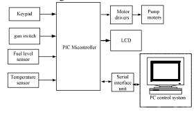
Fig.1 Block Diagram of the System
