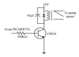
Fig.5 Circuit Diagram of Motor Driver
