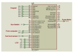
Fig.3 Pin Assignment of the Controller
