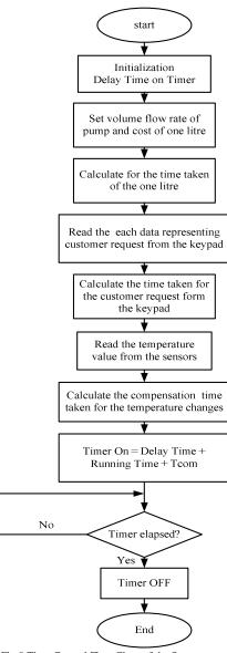
Fig.8 Time Control Flow Chart of the System
