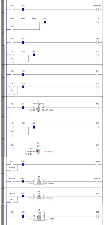
Fig. 3 ladder diagram for biomass gasifier controls
