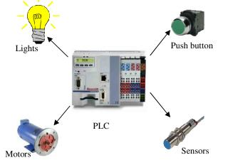
Fig.1. Typical functional components of PLC
