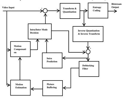
Fig. 2. Block diagram of H.264/AVC encoder
