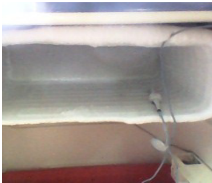
Figure 7: Frost covering the ice formed in an the experiment with 20 litres of water load run 25hrs on a coated evaporator.
