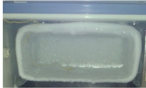
Figure 9: Frost is covering the ice formed in an the experiment with 20litres of water load run 50hrs on a coated evaporator.
