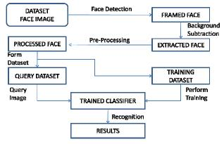
Fig 2. Block Diagram of Face Detection and Recognition System
