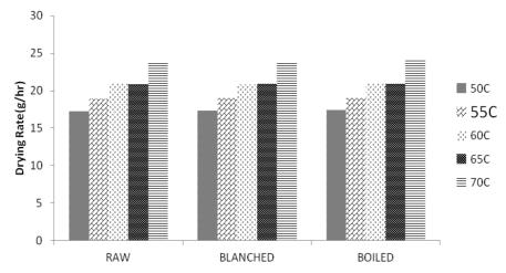
Figure 4. Effect of Pre-Treatment on Drying Rate at different Drying Temperature
