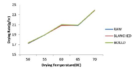
Figure 5. Effect of Pre-treatment on Drying Rate at different Drying Temperature
