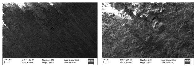
**Fig: 5** Scanning electron microscopy photographs of a porcelain surface treated with diamond bur at 150x,750x showing roughened morphology- peeling and erosive appearance with deeper grooves and undercuts and loss of porcelain structure.
