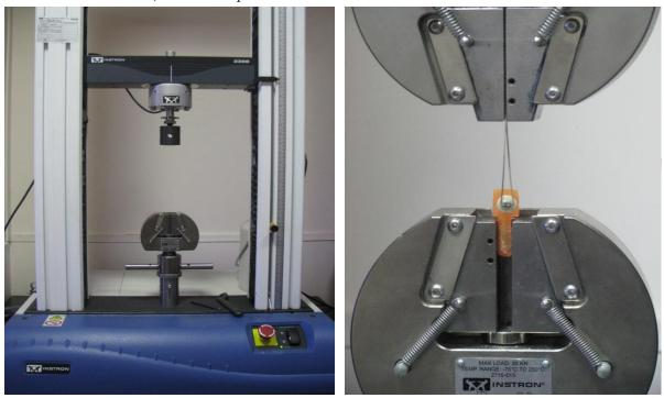
Fig: 1 Instron / Universal testing machine model no 3366 (instron corporation.) Shear bond strength testing
