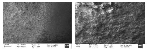
**Fig: 3** Scanning electron microscopy photographs of a porcelain surface treated with sandblasting at 150x,750x showing uniform peeling with shallow undercuts on the porcelain surface
