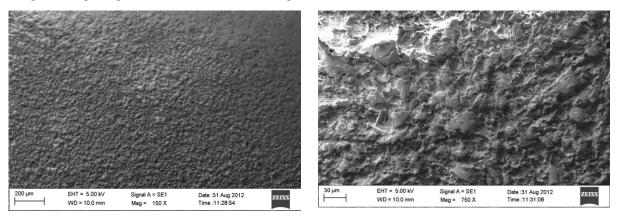
Fig: 4 Scanning electron microscopy photographs of a porcelain surface treated with hydrofluoric acid at 150x,750x showing pits with deeper undercuts and more loss of glazed surface
