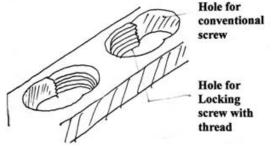
Fig. 4: Locking plate showing combiholes
