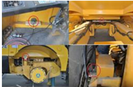
Fig.6 - Sensors placed on the vehicle
