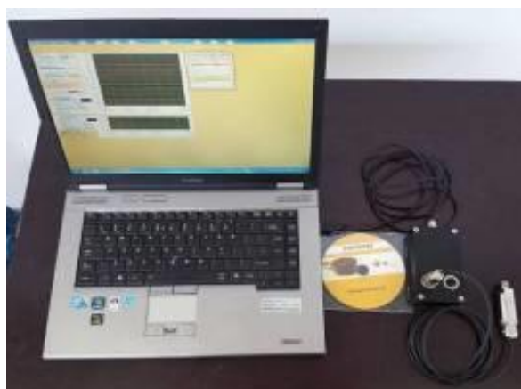
Fig. 2 - Measuring instruments for UV-C radiation intensity
