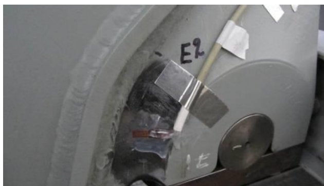
Fig. 3 – Detail of strain gauge application
