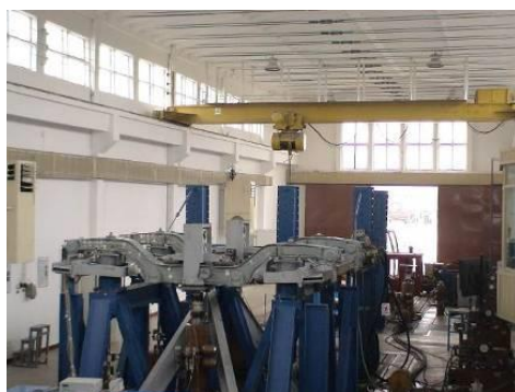
Fig. 5 – Mounting made on the Hydropulse type installation for carrying out the dynamic fatigue tests
