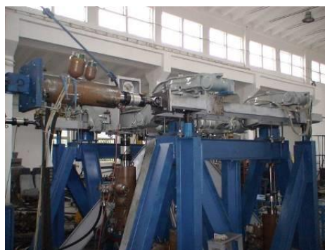
Fig. 5 – Mounting made on the Hydropulse type installation for carrying out the dynamic fatigue tests
