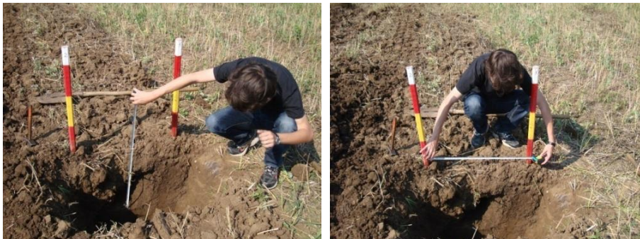
Fig.3 - The transverse section shape of the soil displaced by a plowshare
