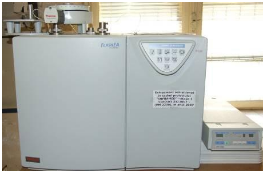
Fig. 7 – Elemental analyzer / Analizor elemental ThermoFinnigan Flash EA 1112
