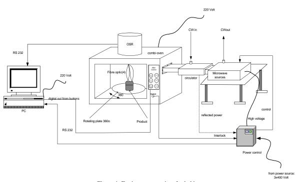
Figure 1. Equipment overview for baking
