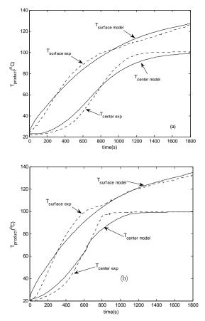
Figure 3. (a) Product temperature during baking experiments (dashed line) and for model calculations (solid line) with convective heating and (b) the combination of convective and microwave heating
