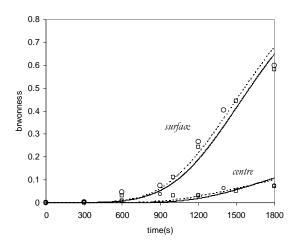
Figure 8. Color developments during baking in the center of the product and at the crust. Results for convective heating ( $\Box$ : experiment; solid line: model) and combined microwave–convective heating (O: experiment; dashed line: model)
