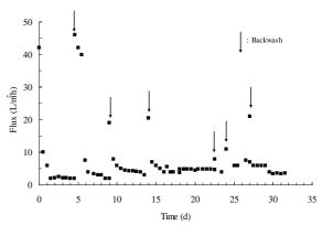
Figure 6. Effect of backwash on MF permeate flux  $(\rightarrow: backwash)$
