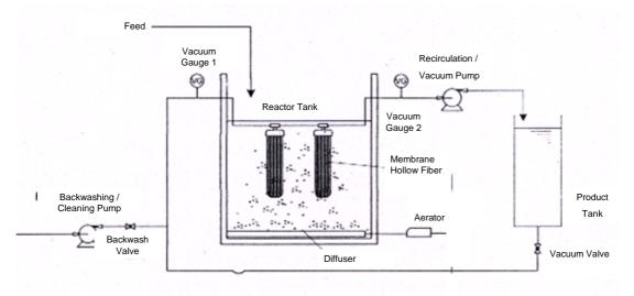
Figure 3. Schematic diagram of UF-MBR for treatment of pulp and paper mill effluent
