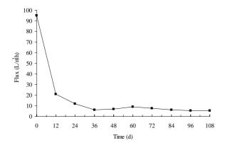
Figure 5. Permeate flux of the microfiltration membrane (leachate)
