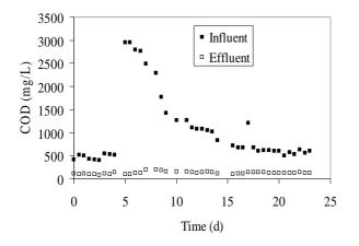
Figure 7. Performance of UF-MBR for treating pulp and paper mill effluent
