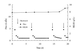
Figure 8. Permeate flux profile of UF membrane (pulp and paper mill effluent)
