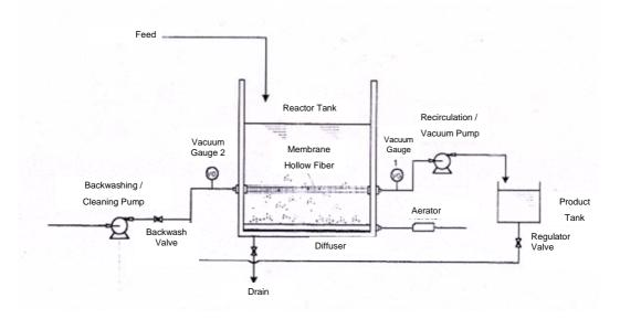
Figure 2. Schematic diagram of MF/UF-MBR for treatment of leachate
