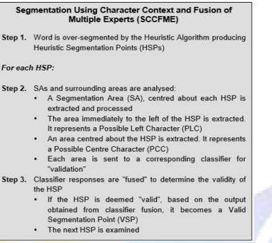
Fig 3.Overview of procedure for segmentation using character context and fusion of multiple experts
