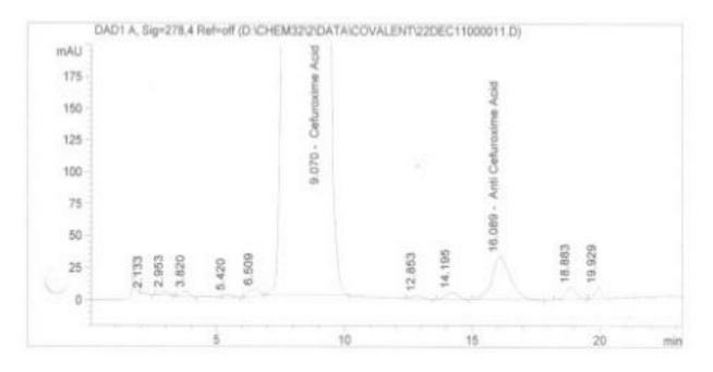
Fig 4: Typical Preparative Chromatogram of Anticefuroximic Acid
