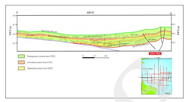
Figure 3. Section of onlap TST MM-1 to the peak of Early Miocene deposition (orange horizon) at seismic line AD-11 showing rising of sea level.
