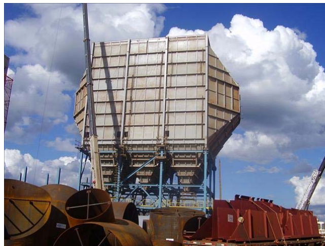
Figure 8 Electrostatic Precipitator in Iron SA (photo of the author's field visit)
