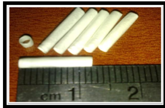
Fig. 1. Display of about 12-mm PLGA/ Nanosilver conduits intended to substitute a 10mm nerve gap.
