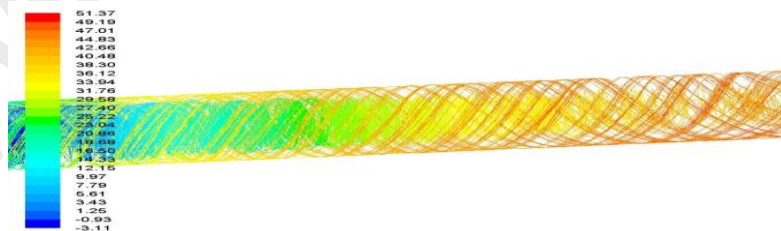
Fig 13 Energy Separation In The Vortex Tube L/D=5.39
