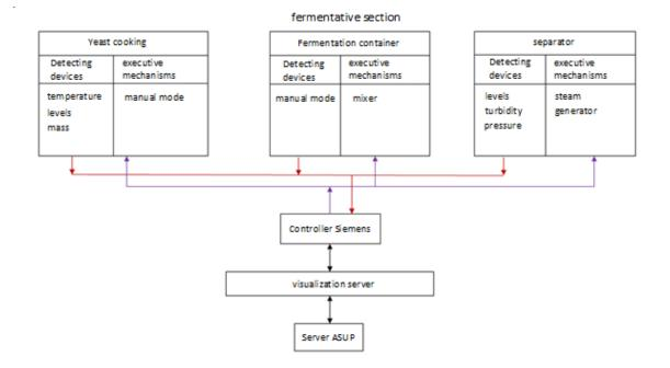
Figure 2 - Block diagram of fermentative section.
