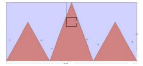
Fig. 3. Triangular shape microstrip antenna.
