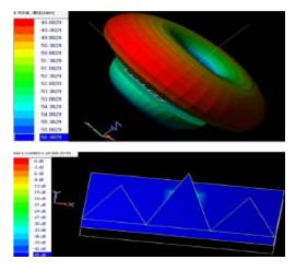
Fig. 6. Radiation pattern & current distribution.
