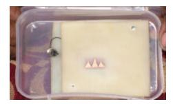
Fig. 2. Photo of triangular shape microstrip antenna.
