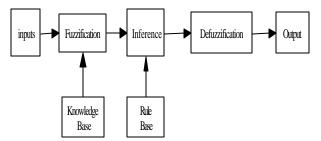
Fig. 1. Block diagram of typical fuzzy logic system and the general inference process.
