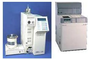
Figure 5: Pictorial View of the Headspace Sampler and GC – FID Used for Aroma Analysis
