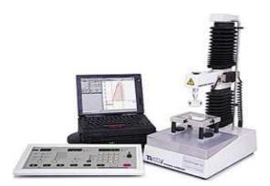
Figure 4: Pictorial View of a Texture Analyser (Model TA- XT2i, Stable Microsystems Ltd. UK)
