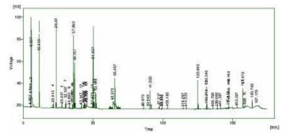
Figure 7: GC – FID Chromatogram for Aroma Volatiles
