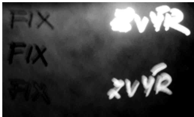
Figure 3. Felt pens (left) and highlight pens (right) under the UV lamp.
