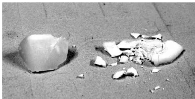
Figure 2. Urea-formaldehyde resin with (left) and without (right) a curing agent after the blow.
