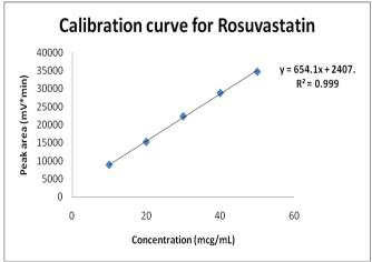
Fig. 2: Calibration curve for ROS
