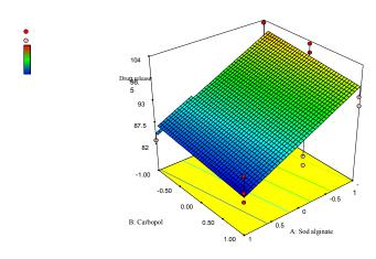
Fig. 4A: Response surface plot showing the effect of carbopol (X1)and Sodium alginate (X2) on drug release
