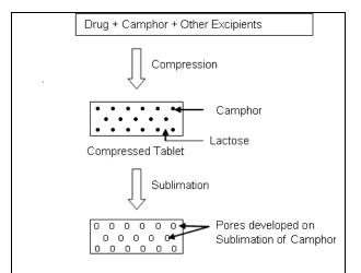
Fig. 1: Schematics figure of Sublimation method for design of Mouth dissolving tablets
