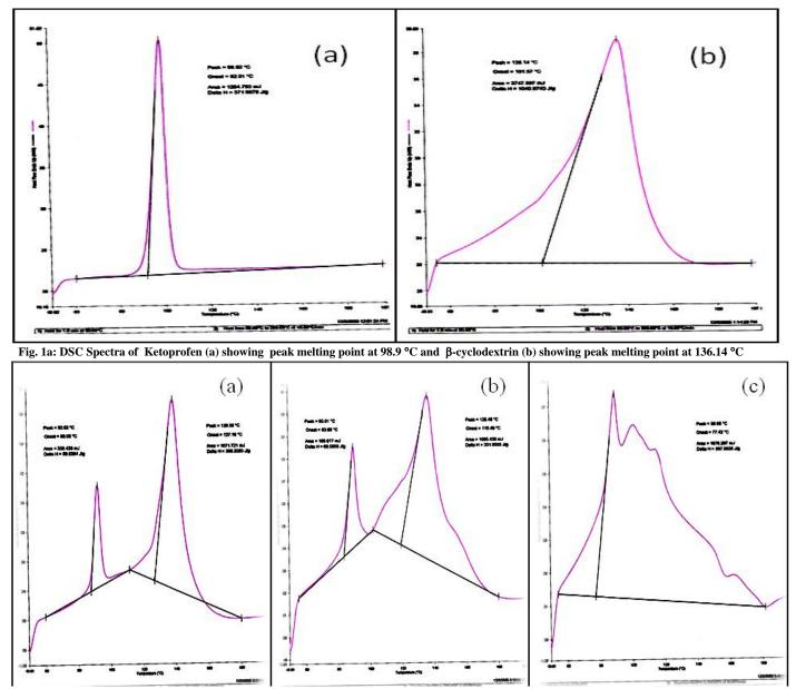
Fig. 1b: DSC Spectra of ketoprofen with β-cyclodextrin prepared by various methods: a. Physical Mixture, b. Kneaded Complex, c. Co-precipitated Complex
