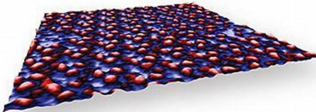
*Figure 7.* Artificial membrane from BR-containing PM in scanning electron microscope (SEM): scanning area – 100 × 100 nm, resolution – 50 nm, magnification – 100000 times. PM shown in purple, BR – in red color
