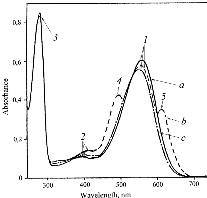
*Figure 8.* The absorption spectra of the PM (50% (v/v) ethanol) at various stages of processing: (a) – natural BR; (b) – PM after intermediate treatment; (c) – PM purified from carotenoids. The bandwidth (1) is the spectral form of BR<sup>568</sup>, (2) – impurity of spectral form of metabacteriorhodopsin (M<sup>412</sup>), (3) – the total absorption bandwidth of aromatic amino acids, (4) and (5) – extraneous carotenoids. As a control used the native BR
