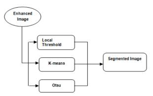
Fig. 3- Segmentation block diagram
