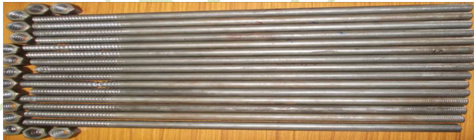
Fig: 2. specimens of mild steel IS2062 tie rods
