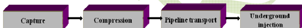
Fig. 2 Schematic presentation showing the major steps in the Carbon Capture and Storage Process
