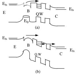
Figure 13 The Energy-band diagrams of the transistor at (a) High-voltage low-current OFF state, (b) Low-voltage high-current ON state
