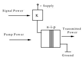
Figure 1 Schematic diagram of a SEED. The n-i-p device is MQW consists of  $GaAs/Al_xGa_{1-x}As$  materials
