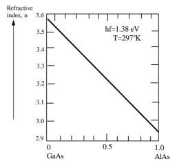
Figure 4 Mole fraction AlAs, x. dependence of index of refraction of  $Al_xGa_{1-x}As$  on the amount of aluminum
