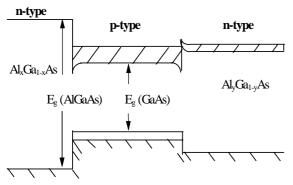
Figure 5 The band diagram for a forward-biased heterostructure
