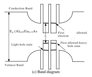
Figure 12 (a) Aluminium concentration as a function of depth in the junction, (b) and (c) the effect of aluminium concentration on the index of refraction and the band gap
