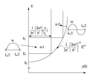
Figure 8 Density of states in a quantum well of thickness  $L_{\rm z}$
