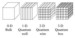
Figure 14 The material structure for bulk, quantum well, quantum wire, quantum box layers
