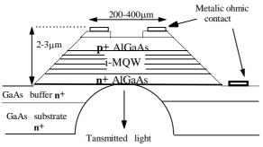
Figure 16 Typical structure of a MQW transmission modulator
