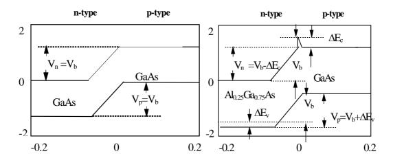
(a) (b) Figure 2 (a) Energy-band diagram for a GaAs n-p homojunction. (b) Energy-band diagram for an  $n-Al_{0.25}Ga_{0.75}As$  /p-GaAs) heterojunction
