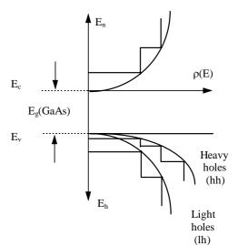
Figure 10 Energy-band structure of GaAs/AlGaAs quantum well
