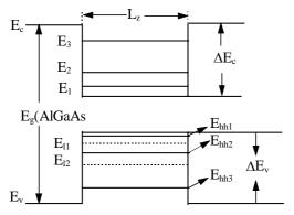
Figure 9 Energy-band structure for a GaAs/AlGaAs heterostructure single quantum well
