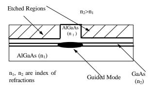
Figure 7 Schematic of the rib waveguide structure. The GaAs active region is sandwiched by AlGaAs cladding layers.
