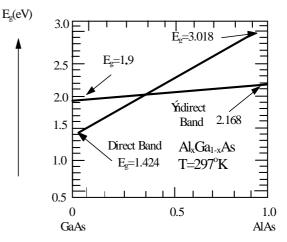
Figure 3 Mole fraction AlAs, x . Dependence of band gap
