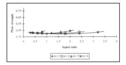
Figure 7. Variation of plate strength against aspect ratio for plates with  $\beta = 3$  and w  $(\delta_0) = 1.38 \, \text{mm}, 3.174 \, \text{mm}, 4.0 \, \text{mm}$
