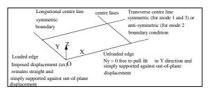
Figure 3 Boundary conditions of a quarter of a plate
