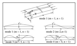
Figure 2. Plate geometry and assumed mode shapes of initial out-of-flatness
