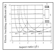
Figure 6. Variation of plate strength against aspect ratio for plates with  $\beta=3$  and  $\delta_0=0.1t\beta^2$
