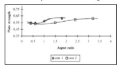
Figure 9. Variation of plate strength against aspect ratio for  $\beta = \frac{b}{t} \sqrt{\frac{\sigma_0}{E}} = 1.92$ ,  $\delta_0 = 0.1t\beta^2$  ase 1 (mode 1+3 and Case 2 (mode 2+4) Plates
