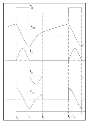
Figure 2. Operational waveforms for the single switch resonant inverter. ( $V_{GS}$ -Gate pulse of the thyristor,  $V_{CrL}$ -Voltage across the load resonant capacitor,  $I_S$ -Thyristor current,  $I_D$ -Diode current,  $V_{LrL}$ -Load voltage)
