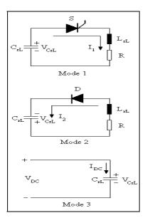
Figure 3. Equivalent modes of operation
