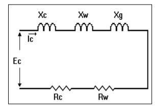
Figure 5. Electrical equivalent circuit of an induction heater coil
