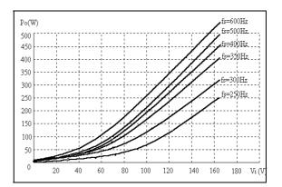
Figure 9. Output power of the induction heating system at different inverter operation frequencies.
