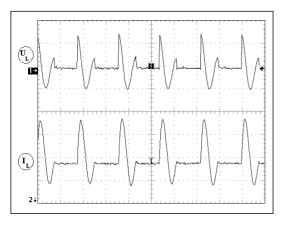
Figure 8. Measured load voltage  $v_L$  and load current  $i_L$  [CH1:50V, CH2: 5A, T: 0.5mS]
