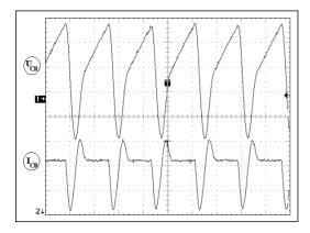
Figure 7. Measured current and voltage waveforms of the load resonant capacitor [CH1: 50V, CH2: 5A, T: 0.5 m S].
