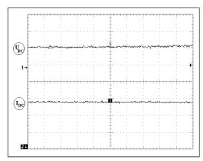
Figure 6 Measured input DC line voltage [CH1:100V, CH2:1A, T:20µS].
