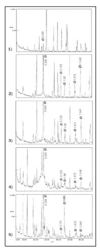
Figure 3. X-ray diffractograms of graphitization material from Tepeköy (1), Tatköy (2, 3) and Meydanköy (4, 5)
